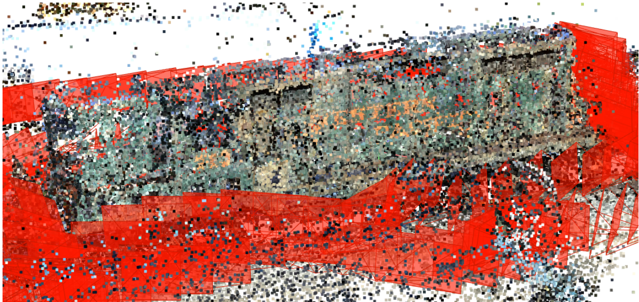
Figure 10: A generated point cloud of a train car using the COLMAP. The red boxes represent camera/picture locations.
